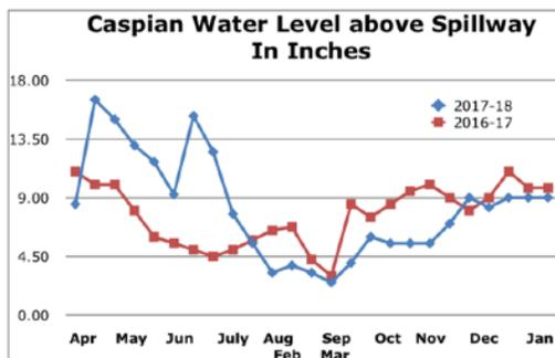
The chart above shows that in the month of January after the gate was opened, the lake level at the spillway increased 3.5 inches rather than decreased. Precipitation in January/February was at or below normal levels so it appears that the outflow was inadequate. A possibility we are studying is that the outflow may have been limited by accumulated debris blocking the new one inch opening at the bottom of the gate. Raising the gate one inch also restricted overflow at the top of the gate.
